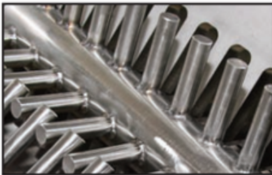
Evenly spaced impacting fingers and replaceable combs on the side walls
